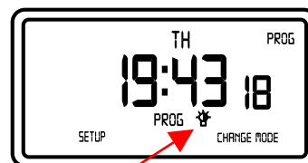
Temporary Override OFF
