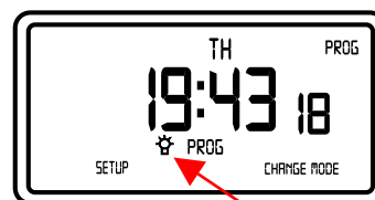
Temporary Override ON
